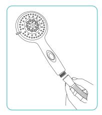
6. Make sure all connections are tightened down and test installation with all spray settings before use.
