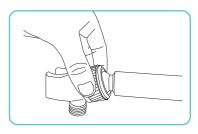
4. Connect the end of the shower hose to the holder bracket. For a tighter seal, it's recommended to add 2–3 layers of thread tape to the bottom end of the mounting bracket.
