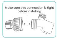
3. Install the mounting bracket to the existing water pipe.
